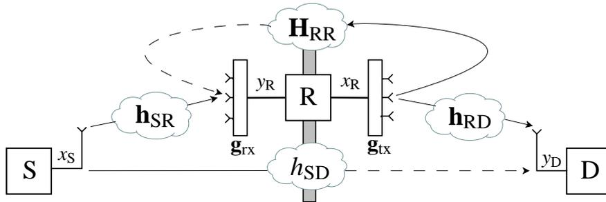
Fig. 1: System model of a two-hop communication system with a full-duplex MIMO relay
