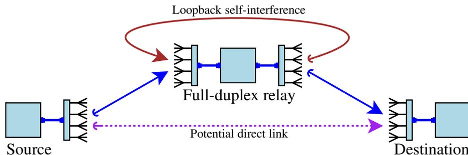
Fig. 1: Two-hop full-duplex multiantenna relay link.
