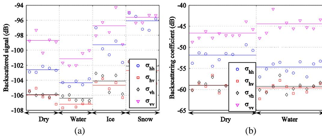
Figure 1. Measured backscattering at different polarizations from: (a) dry, icy and snowy asphalt, (b) dry and wet asphalt. Single measurements are represented with markers and solid lines are averaged values over respective road condition and polarization.
