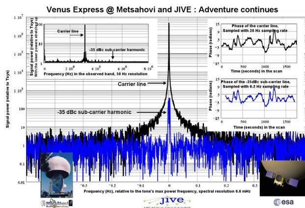
**Figure 2: Results of the Metsähovi, JIVE phase-referenced satellite tracking demo allow GPS-like tracking beyond 100 earth-sun distances.**
