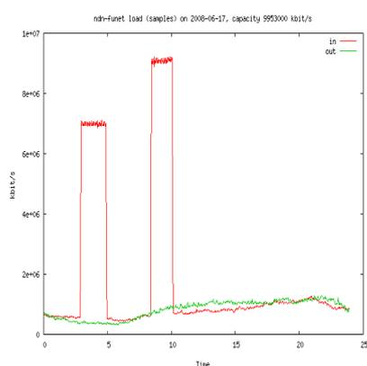
**Figure 1: Real-time Internet data streaming at 6 and 8 Gbps using the Metsähovi system. Plots © Nordunet.**
