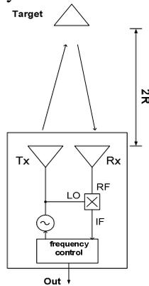
Figure 1: Vibration measurement with a monostatic FM-CW radar [1].
